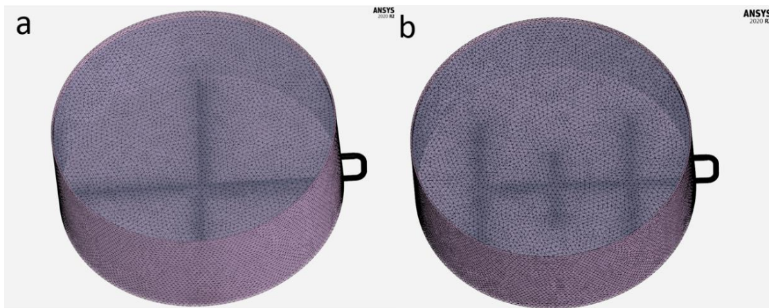
Figure 2. Computational Mesh of 3D Model with (a) Directional Jet Mixer (b) Hydraulic Sludge Mixer
